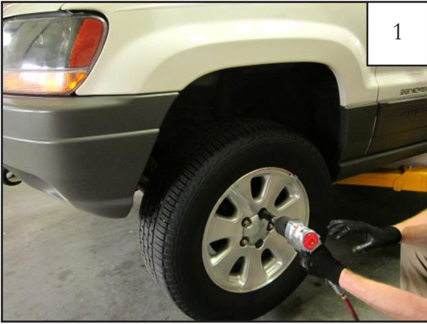
Using a car jack, lift vehicle from the ground and place jack stands under lower control arms to prop up during installation. Remove tire using an impact wrench.
