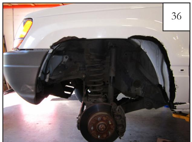
Completed cut-out with caulking applied.
